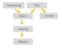
Figure 3: Fire Alarm Inferencing (Bayesian Network) [19]
